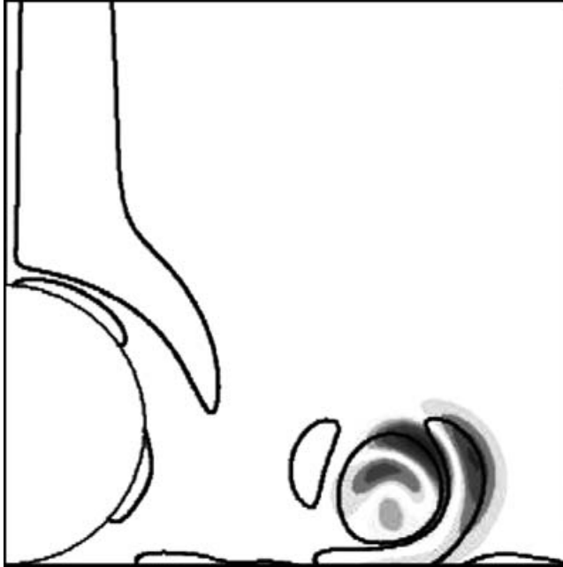
FIGURE 24. Perturbation vorticity distribution of the mode m = 20 for Re = 1200 and L/D = 5 at \tau = 10 , obtained from the three-dimensional simulation. Contours of the azimuthal vorticity field ( m = 0 ) are overlaid to show the location of the primary vortex ring and the secondary vorticity. Note that the vorticity field varies sinusoidally in the azimuthal direction.
